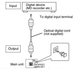
Digital audio signals are output from this system only when DVD/CD is selected as the source.
