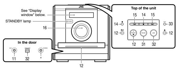
\* Connect headphones (not supplied) with a stereo mini plug. If the headphones are connected, the speakers and subwoofer will not produce any sound.
