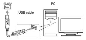
• Use "USB series A plug to B plug" cable (version 1.1 or later) less than 3 m (10.7 ft.).
