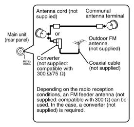
For details of connecting a separately sold antenna, refer to the user guide for the antenna or converter.
