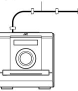
When good radio reception cannot be obtained with the supplied antenna or when using a communal antenna
