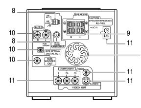
These holes discharge heat generated inside the unit. Do not cover up these holes.
