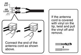
**3** Turn the AM loop antenna to the direction of the best radio reception.
