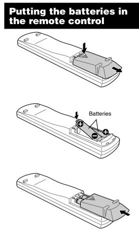
If the range or effectiveness of the remote control decreases, replace the batteries. Use two R6 (SUM-3)/AA(15F) type dry-cell batteries.
