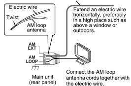
When positioning the antenna, find the best position for reception while listen to an actual radio program (refer to "Listening to a radio broadcast" on page 31).
