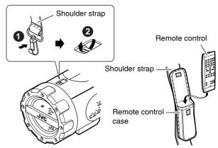
To detach the shoulder strap, press in the metal fitting and unhook it from the shoft
