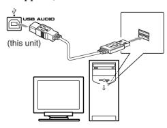
• Use "USB series A plug to B plug" cable when connecting.
