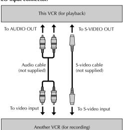
Example 3: When another VCR is S-VHS VCR and when using this VCR as the recording VCR
