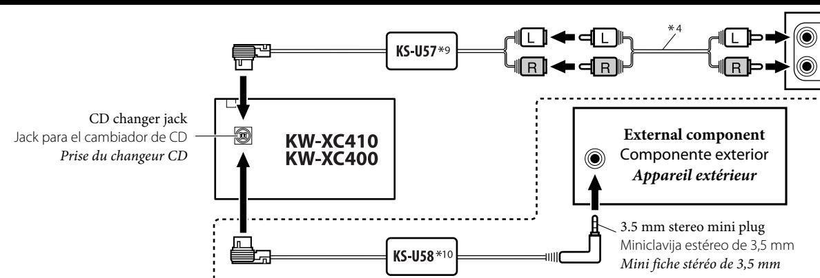
\*<sup>9</sup> Line Input Adapter KS-U57 (not supplied for this unit)
