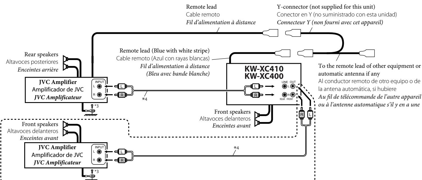
\*3 Firmly attach the ground wire to the metallic body or to the chassis of the car—to the place uncoated with paint (if coated with paint, remove the paint before attaching the wire). Failure to do so may cause damage to the unit.
