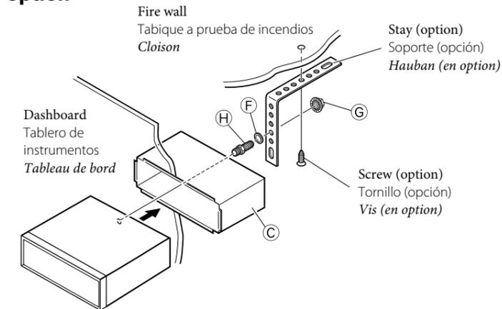
Install the unit at an angle of less than 30°.
