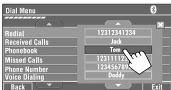
When using the remote controller, you can display <Redial> list anytime (except when Dual Zone is in use).
