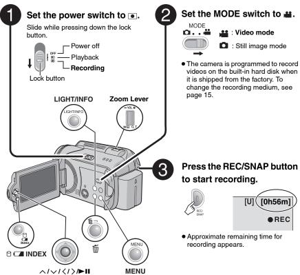
To stop recording Press the **REC/SNAP** button again.
