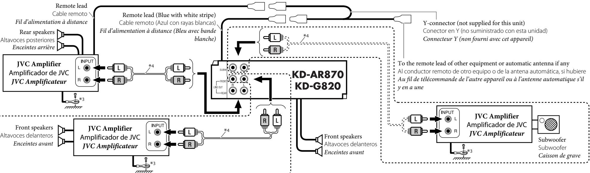
\*3 Firmly attach the ground wire to the metallic body or to the chassis of the car—to the place uncoated with paint (if coated with paint, remove the paint before attaching the wire). Failure to do so may cause damage to the unit.
