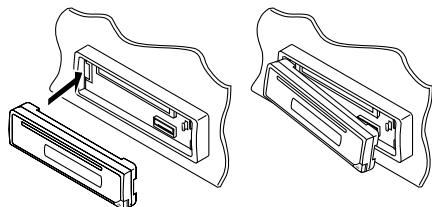
**2** **Press the right side of the control panel to fix it to the panel holder.**
