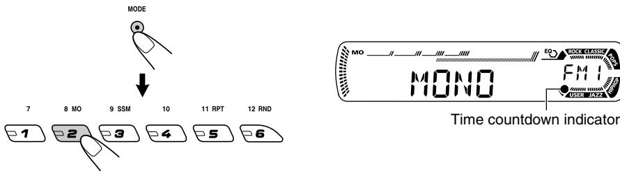
To use these buttons for original functions again after pressing MODE, wait for 5 seconds without pressing any of these buttons until the functions mode is cleared.
