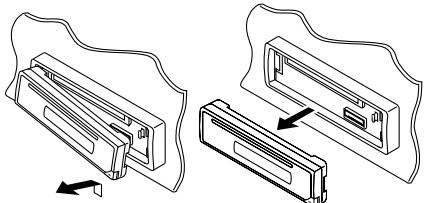
**3** **Put the detached control panel into the provided case.**
