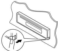
**2** **Lift and pull the control panel out of the unit.**
