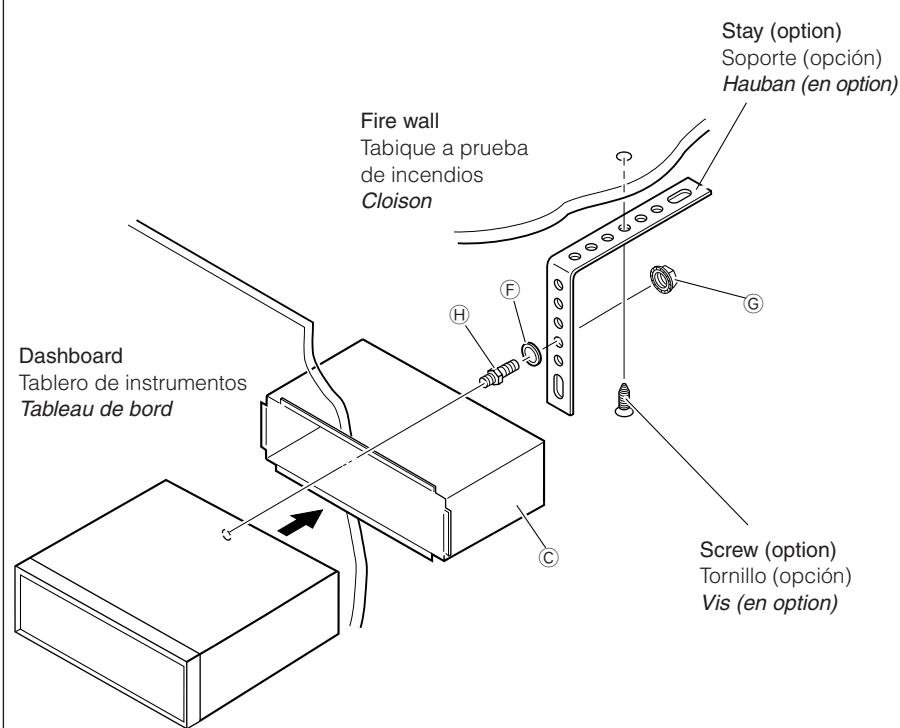
Install the unit at an angle of less than 30°.
