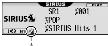
\* Signal strength bar increases as the receiving signal improves. If no signal is received, it disappears.
