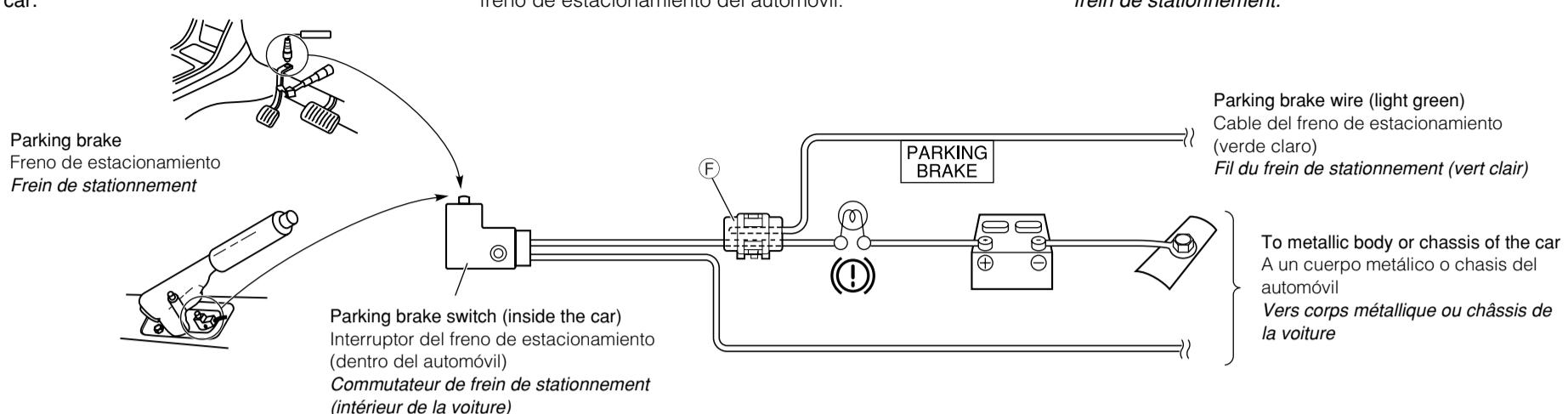
When installing the monitor in a location where it cannot be seen by the driver
