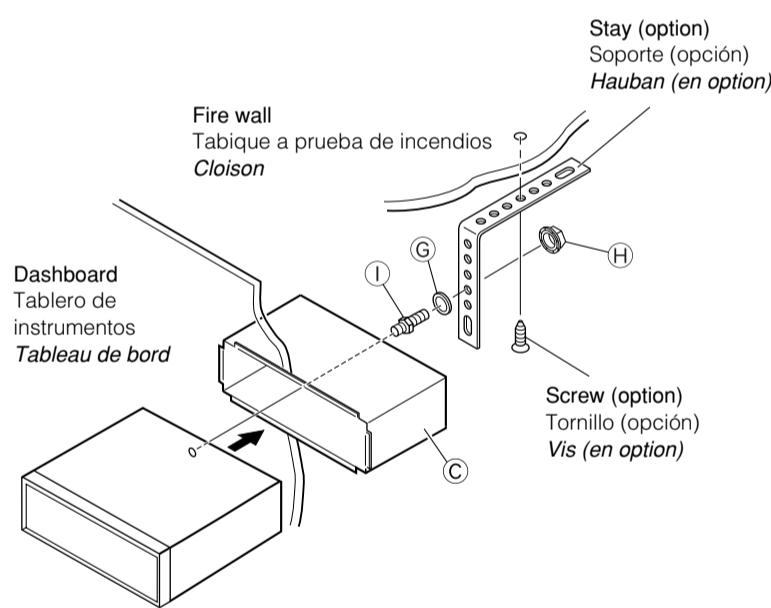
Install the receiver at an angle of less than 30°.
