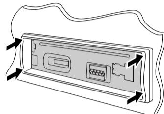
Fit the receiver into the mounting sleeve by using four corners of the trim plate.
