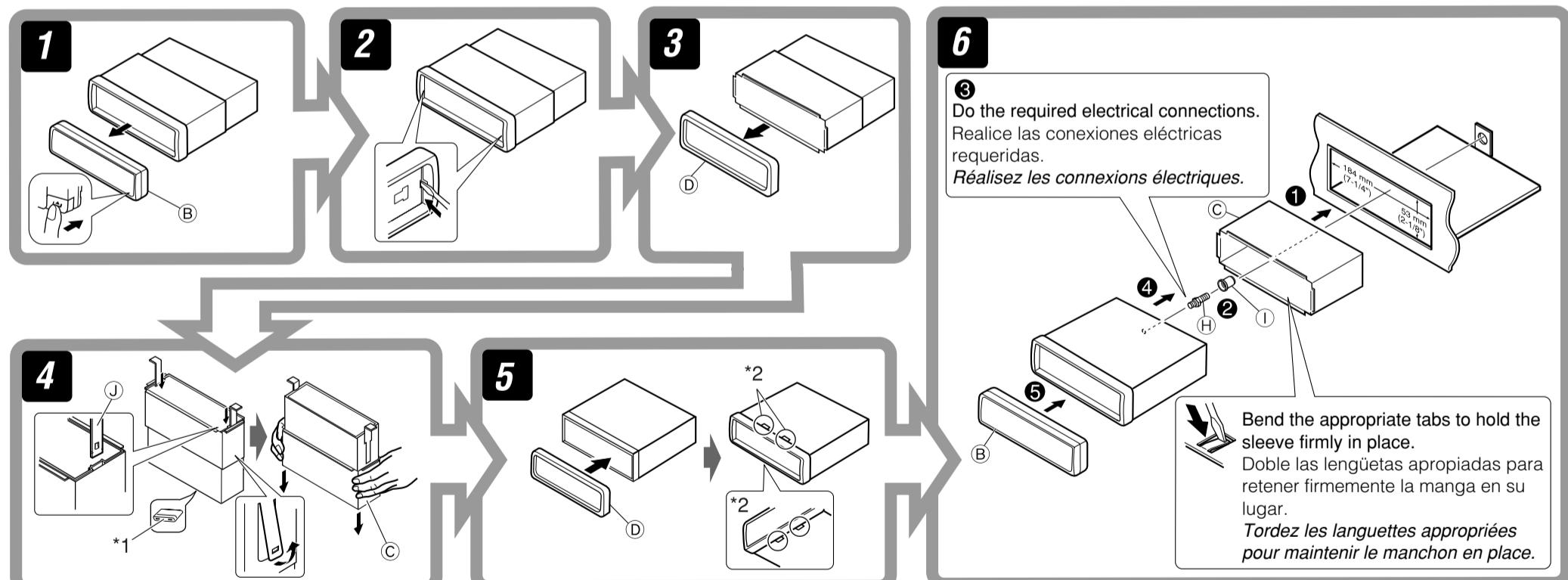
\*1 When you stand the receiver, be careful not to damage the fuse on the rear.
