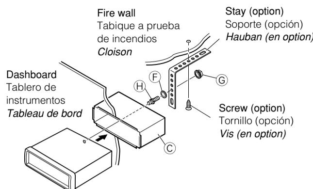
Install the receiver at an angle of less than 30°.
