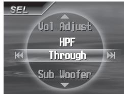
Adjust the cut-off frequency to the front/rear speakers according to the subwoofer setting.
