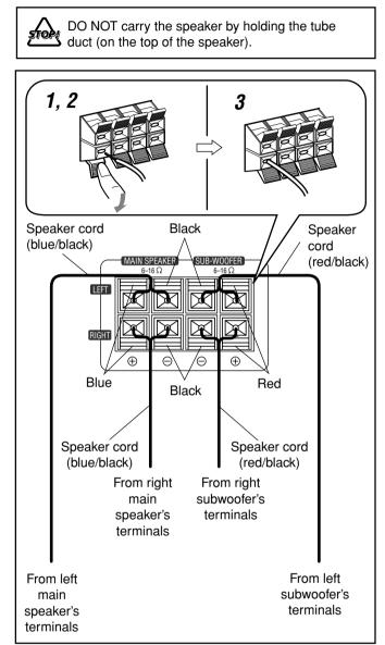
**1** Press and hold the clamp of the speaker terminal on the rear of the unit.
