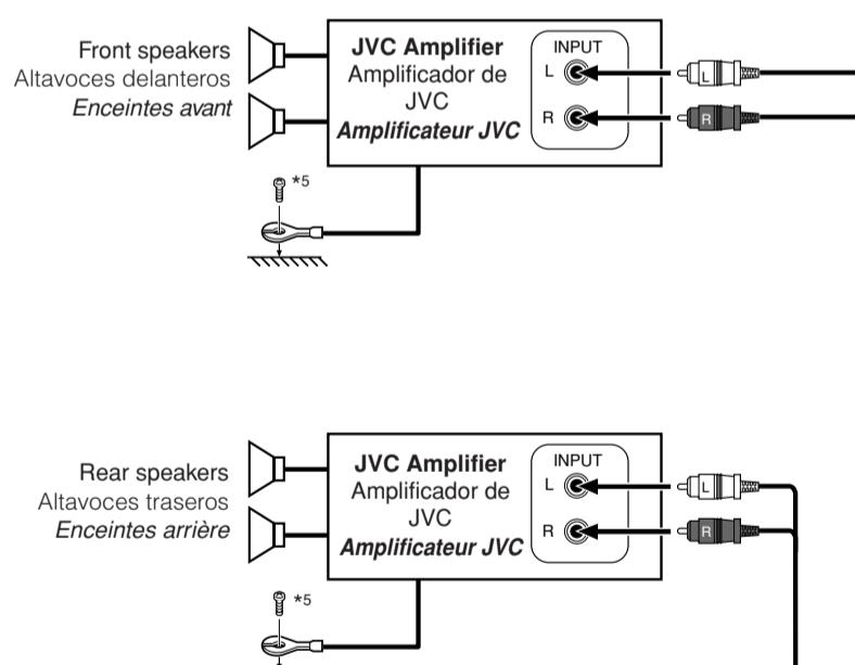
\*5 Firmly attach the ground wire to the metallic body or to the chassis of the car—to the place uncoated with paint (if coated with paint, remove the paint before attaching the wire). Failure to do so may cause damage to the unit.
