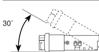
Install the unit at an angle of less than 30°, taking it into account that the monitor would eject when in use (see below).
