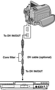
Video unit equipped with DV connector
