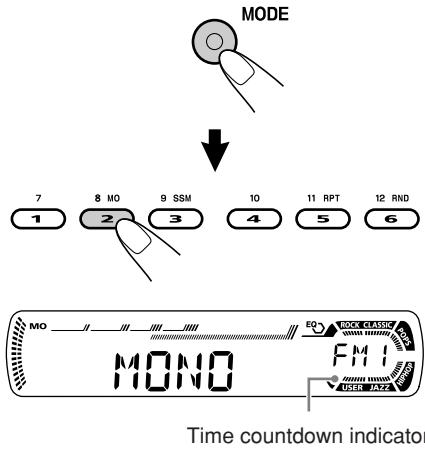
To use these buttons for original functions again after pressing MODE, wait for 5 seconds without pressing any of these buttons until the functions mode is cleared.
