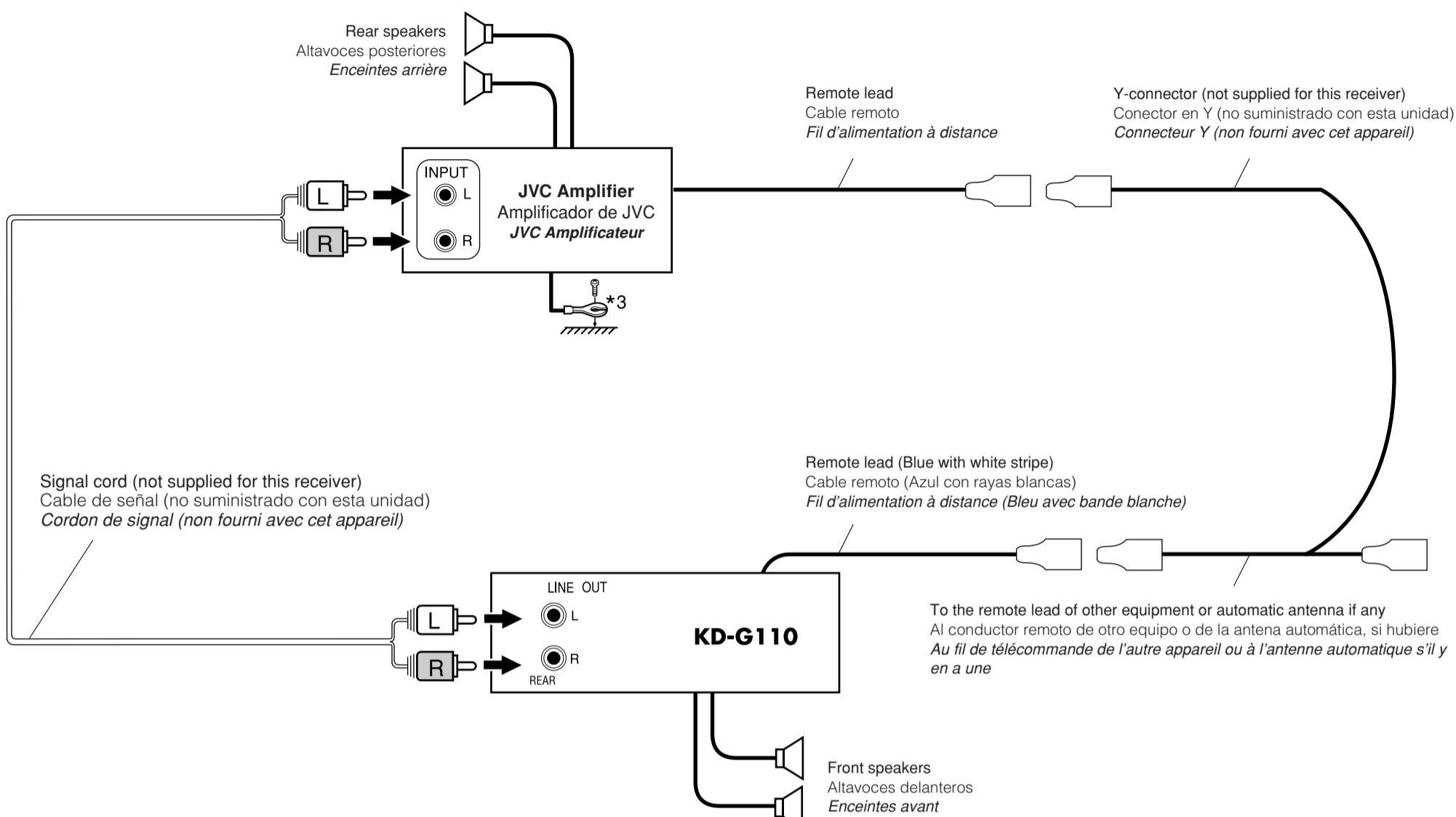
\*3 Firmly attach the ground wire to the metallic body or to the chassis of the car—to the place not coated with paint (if coated with paint, remove the paint before attaching the wire). Failure to do so may cause damage to the receiver.
