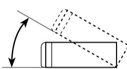
Install the receiver at an angle of less than 30°.
