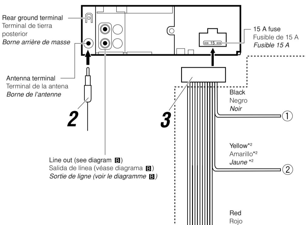
\*<sup>2</sup> Before checking the operation of this unit prior to installation, this lead must be connected, otherwise power cannot be turned on.
