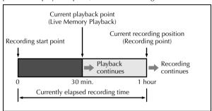
Not only can this unit play back a program previously recorded while recording or timer recording another program, but the unit also allows you to play back from the beginning of a program while continuing to record the same program.
