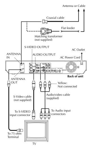
■ To connect to TV's S-VIDEO input and AUDIO input connectors
