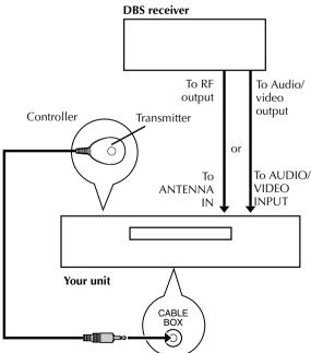
The following procedure is required if you receive satellite channels through a DBS (Direct Broadcast Satellite) receiver. The Controller allows the unit to automatically switch the DBS receiver's channel during timer recording.
