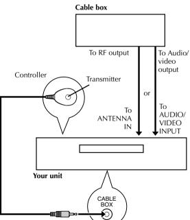
The following procedure is required if you receive your TV channels through a cable box (descrambler). The Controller allows the unit to automatically switch the cable box channel during timer recording. The Controller is effective for recording broadcasts that have been programed using "VCR Plus+\* Timer Programing" (\$\mathbb{C}\$ pg. 60) or "Manual Timer Programing" (\$\mathbb{C}\$ pg. 64).
