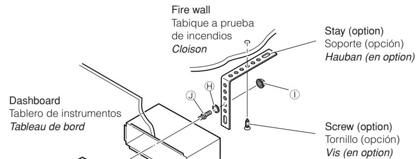
Install the unit at an angle of less than 30°.
