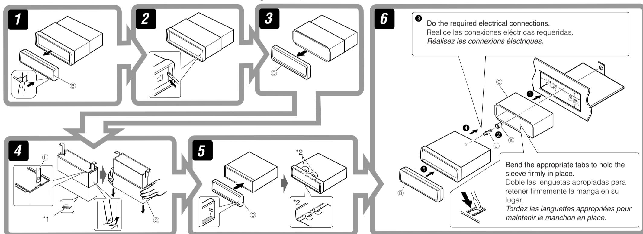
\*1 When you stand the unit, be careful not to damage the fuse on the rear.
