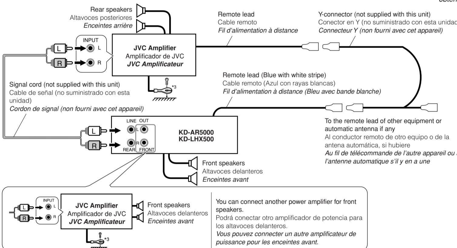
\*3 Firmly attach the ground wire to the metallic body or to the chassis of the car—to the place not coated with paint—if coated with paint, remove the paint before attaching the wire). Failure to do so may cause damage to the unit.
