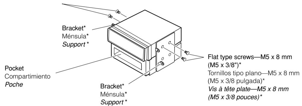
**Note** : When installing the unit on the mounting bracket, make sure to use the 8 mm (3/8") -long screws. If longer screws are used, they could damage the unit.
