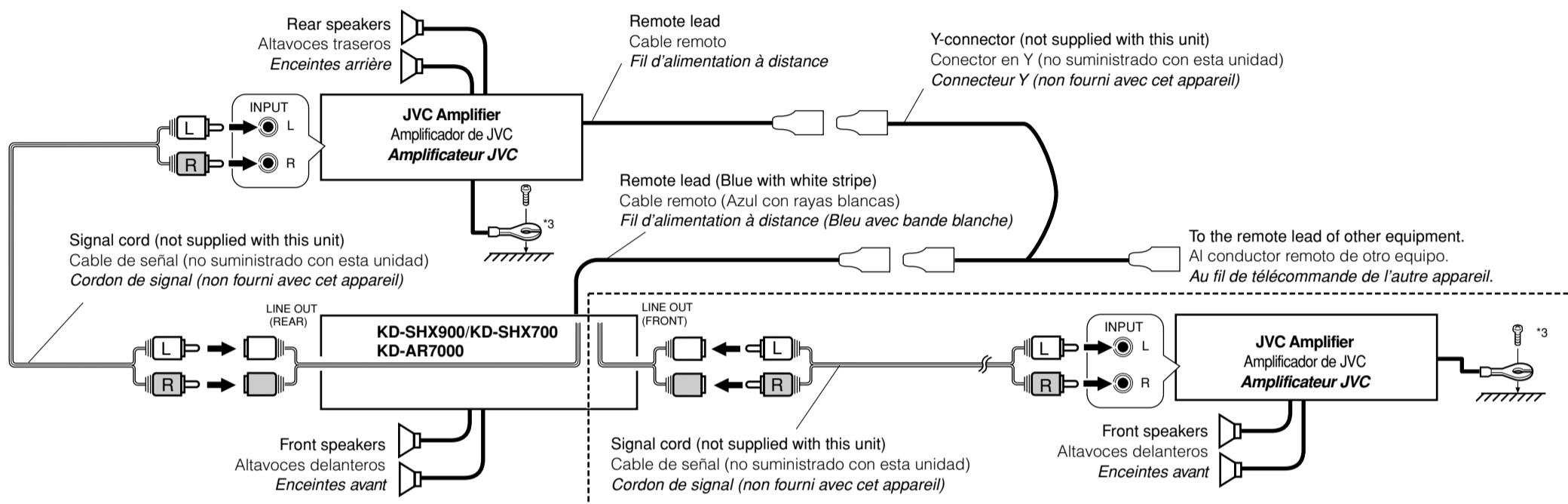
\*<sup>3</sup> Firmly attach the ground wire to the metallic body or to the chassis of the car—to the place not coated with paint, (if coated with paint, remove the paint before attaching the wire). Failure to do so may cause damage to the unit.
