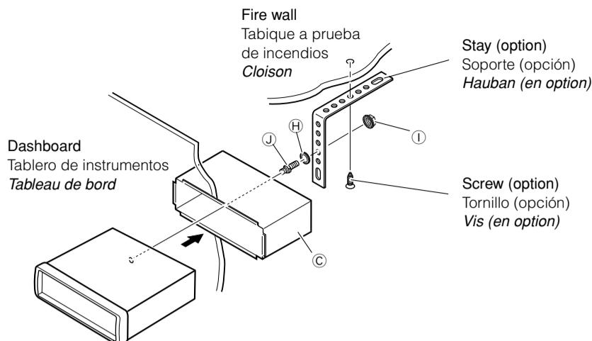
Install the unit at an angle of less than 30°.
