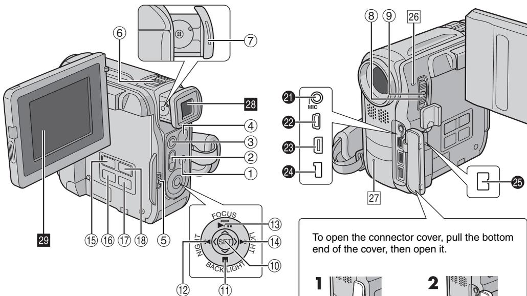
To open the connector cover, pull the bottom end of the cover, then open it.
