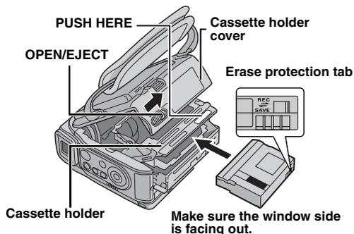
**1** Slide and hold **OPEN/EJECT** in the direction of the arrow, then pull the cassette holder cover open until it locks. The cassette holder opens automatically.
