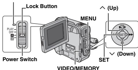
Choose the appropriate operation mode according to your preference using the Power Switch and VIDEO/MEMORY Switch.
