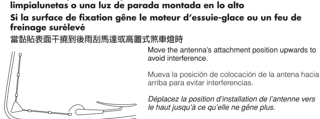
Move the antenna's attachment position upwards to avoid interference.
