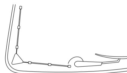
Move the antenna's attachment position upwards to avoid interference.
