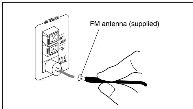
1 Attach the FM antenna to the FM 75 Ω COAXIAL terminal.
