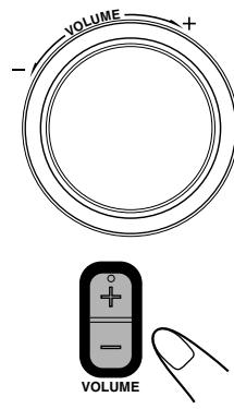
When using the remote control, press VOLUME + to increase the volume or VOLUME – to decrease it.
