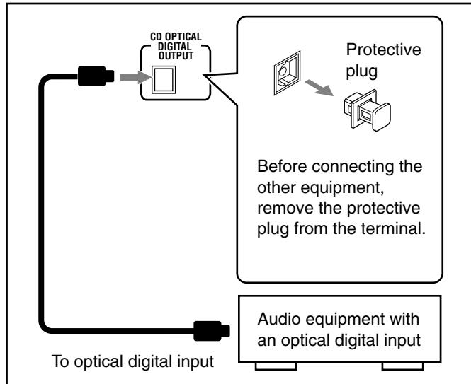
Connect an optical digital cord (not supplied) between the optical digital input terminal on the other equipment and the CD OPTICAL DIGITAL OUTPUT terminal.
