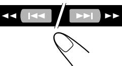
The unit starts searching for stations and stops when a station of sufficient signal strength is tuned in.
