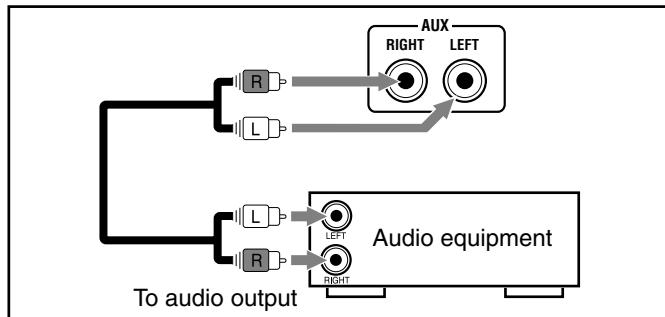
For playing the other equipment through this unit, connect between the audio output jacks on the other equipment and AUX jacks by using an audio cord (not supplied).
