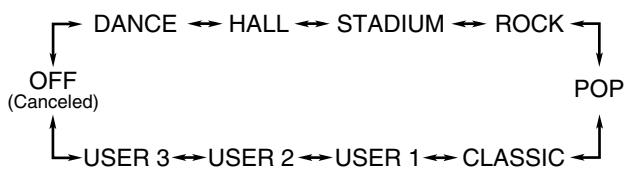
When using the remote control, the sound mode changes only clockwise in the above sequence.
