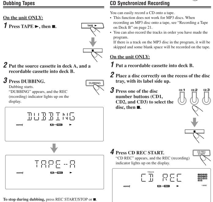
To remove the cassettes, press **A** EJECT for deck A and
