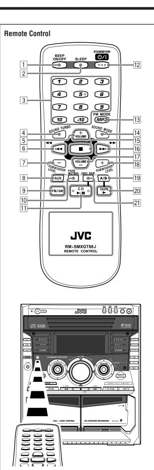
When using the remote control, point it at the remote sensor on the front panel.
