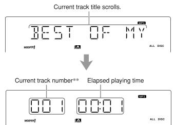
\*\* In the TRACK mode, the unit manage only files (tracks) on the MP3 disc. Folders (albums) are not recognized.
