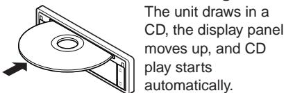
The unit draws in a CD, the display panel moves up, and CD play starts automatically.
