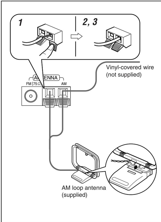
**1** Press and hold the clamp of the AM terminal on the rear of the unit.
