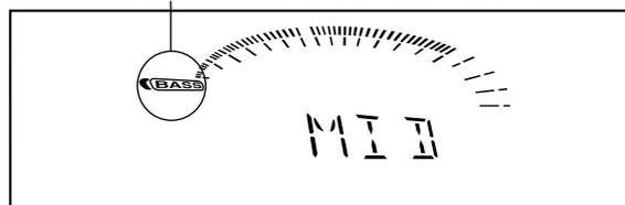
When using the remote control, press **ACTIVE BASS EX. LEVEL** to adjust the bass sound level. Each time you press the button, the Active Bass Extension level changes as OFF → LOW → MID → HIGH → (back to the beginning).
