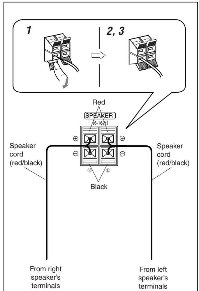
**1** Press and hold the clamp of the speaker terminal on the rear of the unit.
