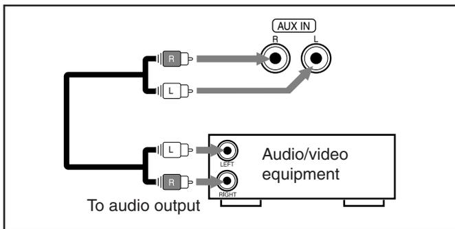
**For playing the other equipment through this unit,** connect between the audio output jacks on the other equipment and AUX IN jacks by using audio cords (not supplied).
