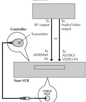
The following procedure is required if you receive your TV channels through a cable box (descrambler). The Controller allows the VCR to automatically switch the cable box channel during timer recording. The Controller is effective for recording broadcasts that have been programmed using VCR Plus+ system (\$\mathbb{C}\$ pg. 30) or Express timer programing (\$\mathbb{C}\$ pg. 34).
