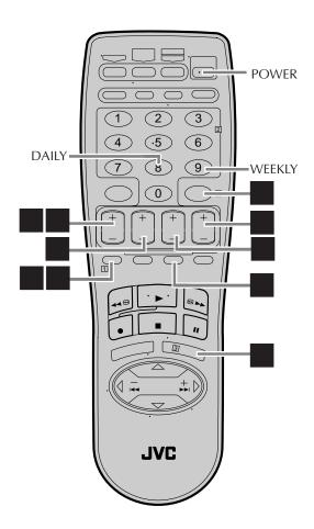
You can directly program the VCR's timer to record up to 8 programmes, as far as a year in advance. Remember, the clock must be set before you can program the timer (pp. 8 or 10).
