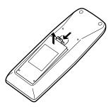
2 Place the two accessory AA (15F), R6, SUM-3 batteries in the remote control making sure to align the polarity markings ("+" and "-") inside the compartment and on the batteries.
