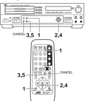
1 When the unit is in stop mode, press the MENU button (or the DISPLAY/MENU button on the remote control while holding down the SHIFT button).
