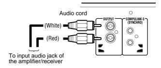
If you are connecting the unit to a JVC audio component and using the CompuLink-3 remote control system, connect the units with the accessory CompuLink cord. Either one of the COMPULINK-3 (SYNCHRO) ports in the back of this unit can be used.
