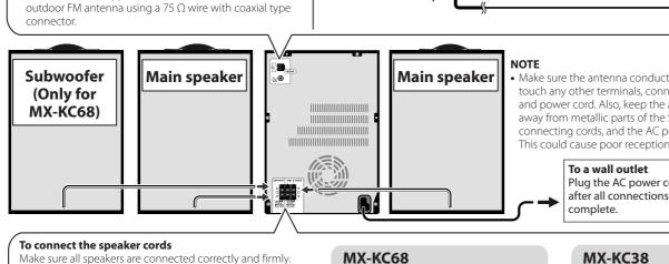
Make sure all speakers are connected correctly and firmly. When connecting the speaker cords, match the polarity of the speaker terminals:
