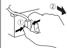
Hold the connector top tightly (1), then pull it out (2).
