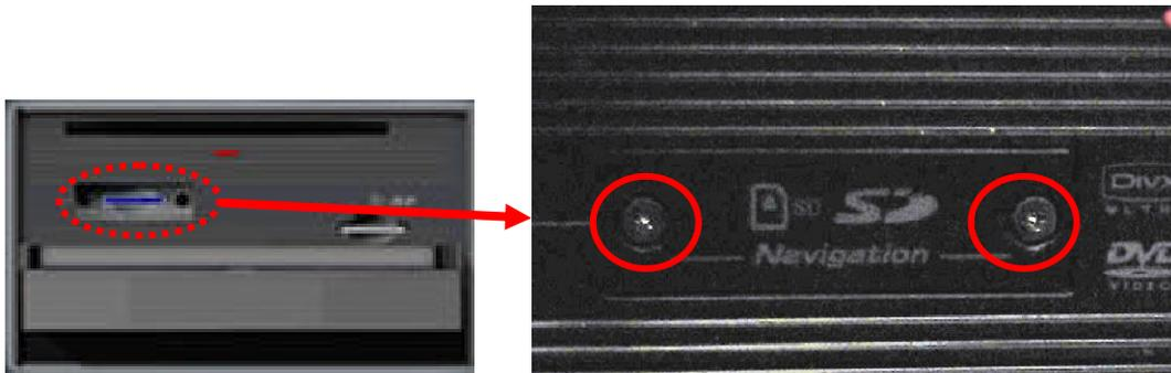
2-8. Insert the SD card created in procedure 1 into the left slot. When the SD card is inserted, the display changes as shown below. Touch [OK] as indicated.
