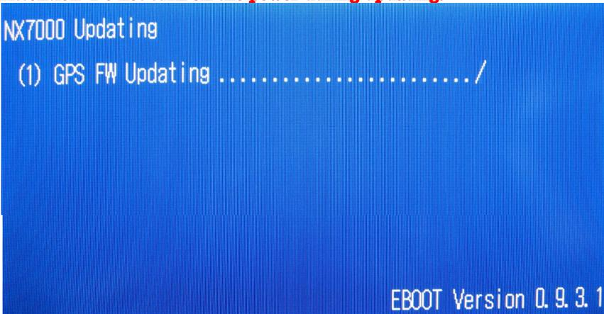
If the screen shows “Retry” or “Fail”, remove the SD card from the unit and press the reset button located next to the power (ATT) button. When the unit restarts, power the unit ‘OFF’ and turn ‘OFF’ ignition key. After turning ignition “ON” reattempt the firmware procedure. If you have any operational questions or issues after this update, please contact JVC Customer Care Center or JVC Service Center.
