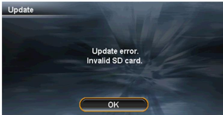
2-14. Eject the SD card and attach the slot cover removed in procedure 2-7 Touch [OK].
