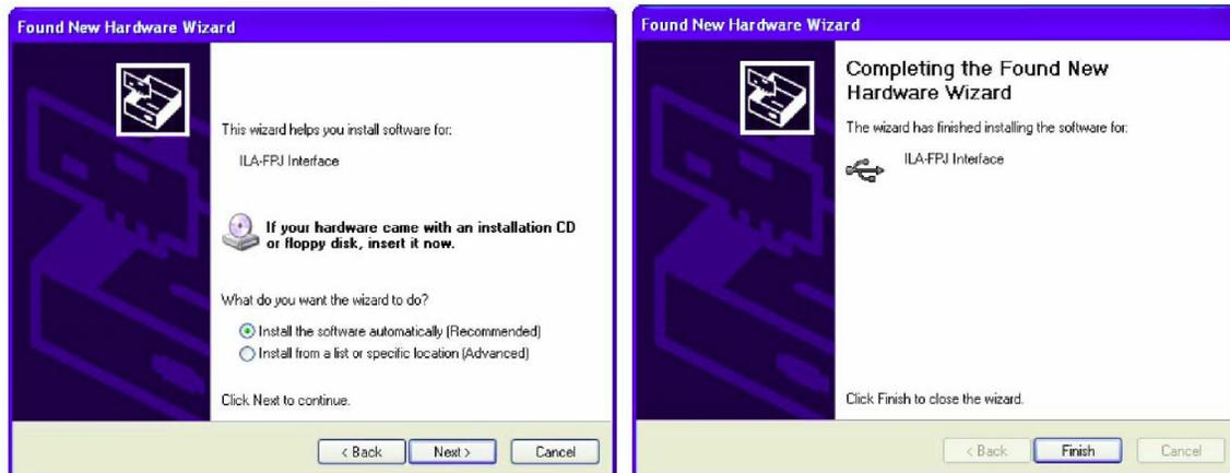
9. The driver will be installed and a confirmation message is displayed that the installation is finished.
