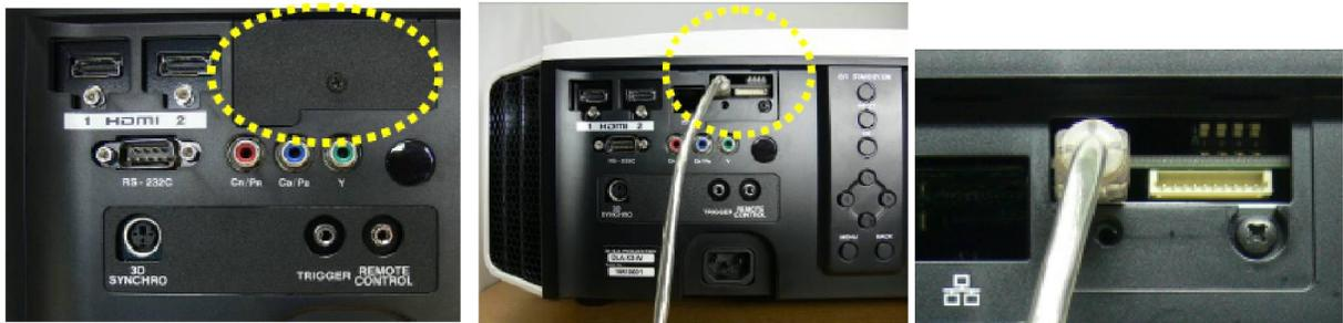
4. Connect PC to Projector using the USB cable as shown above.
