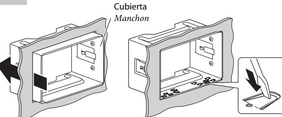
Bend the appropriate tabs to hold the sleeve firmly in place.
