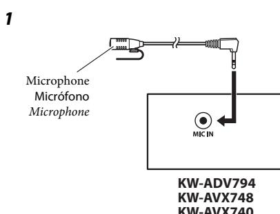
Secure the microphone cord using cord cramps (not supplied) if necessary.
