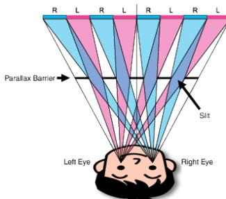
3D images on the LCD monitor of this unit are displayed using the parallax barrier system. Placed in front of an image source, a parallax barrier consists of a series of slits arranged alternately for the left and right eyes, allowing each eye to see a different image when viewing from a distance, thus creating the 3D effect. As such, 3D effect may appear weak depending on the angle of viewing.
