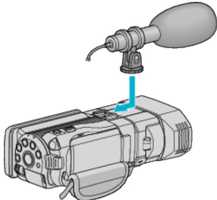
2 Open the cover of the microphone connector and connect the cable of the external microphone.
