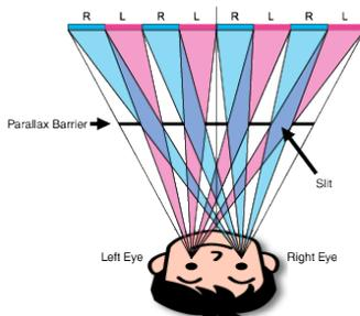
3D images on the LCD monitor of this unit are displayed using the parallax barrier system. Placed in front of an image source, a parallax barrier consists of a series of slits arranged alternately for the left and right eyes, allowing each eye to see a different image when viewing from a distance, thus creating the 3D effect. As such, 3D effect may appear weak depending on the angle of viewing.
