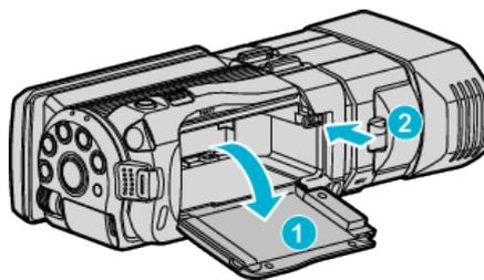
Press the battery release lever to detach the battery from this unit.
