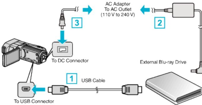
1 Connect the USB cable of the external Blu-ray drive to this unit.
