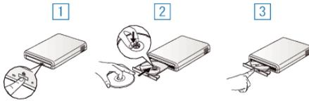
1 Press the eject button to open the disc tray.
