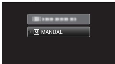
6 Adjust the focus with the UP/< and DOWN/> buttons.
