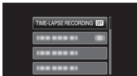
3 Select a recording interval (1 to 80 seconds) and press OK.
