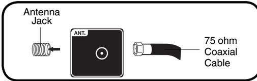
Connect the 75 ohm cable from the combination VHF/UHF antenna to the Antenna Jack.
