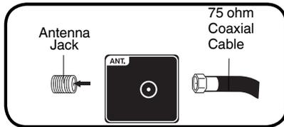
For basic Cable TV service not requiring a Converter/Descrambler box, connect the 75 ohm Coaxial Cable directly to the Antenna Jack on the back of the TV.
